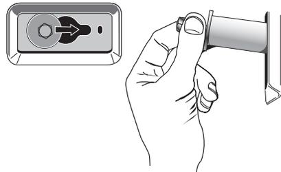
4. Once all 4 bolts are removed, discard the bolts and spacers. Then push the power cord plug into the opening on the right side of the rear panel and pull the power cord through the opening on the left side of the rear panel and close holes with the attached cap. Do not pull plug end of power cord through the right side hole.
